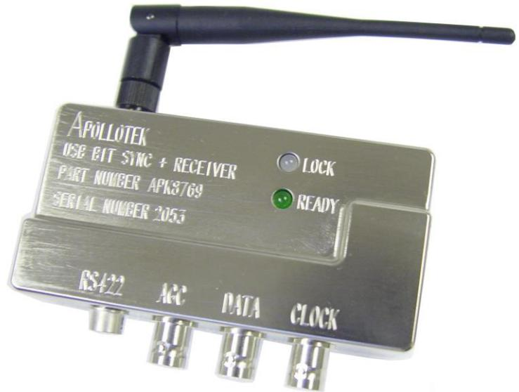
The Apollotek APK8769 incorporates an S-Band or L-Band Telemetry Receiver with an integral Bit Synchroniser and is one of the Apollotek range of USB products which are designed for PCM Flight Test Instrumentation system evaluation and test applications.
